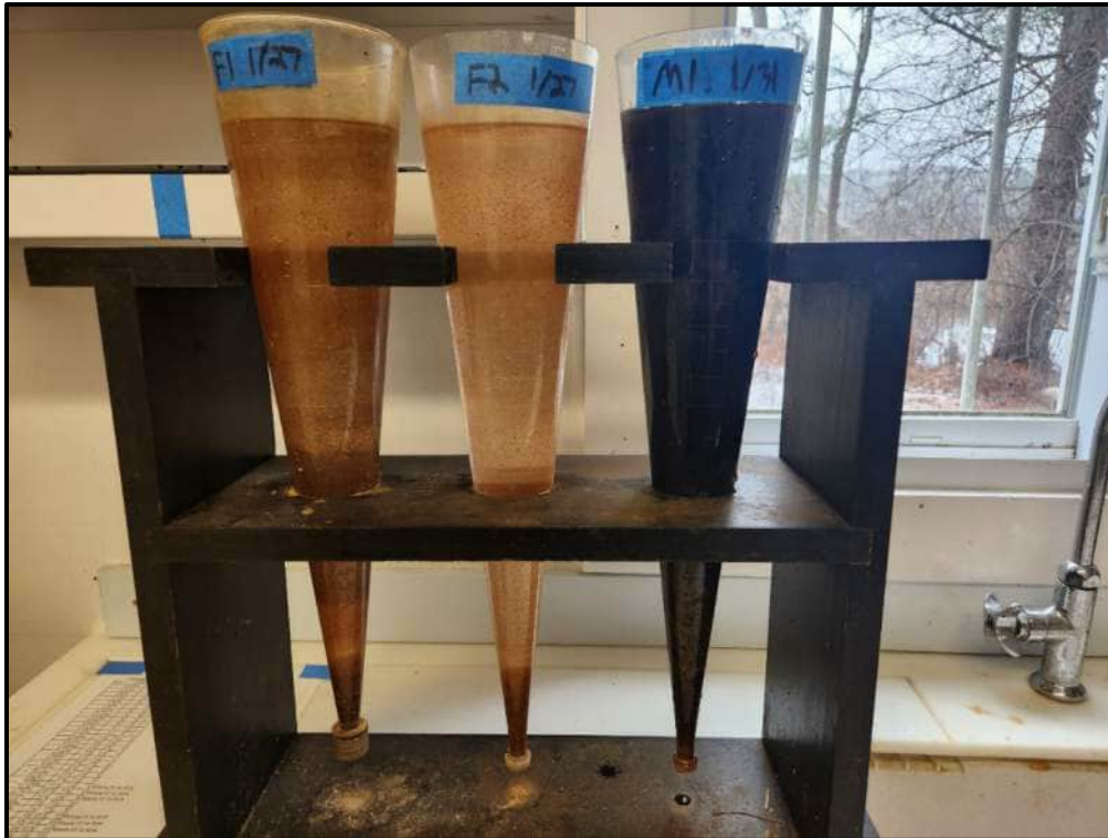
Figure 3.07: Photo of Imhoff Settling Cones
