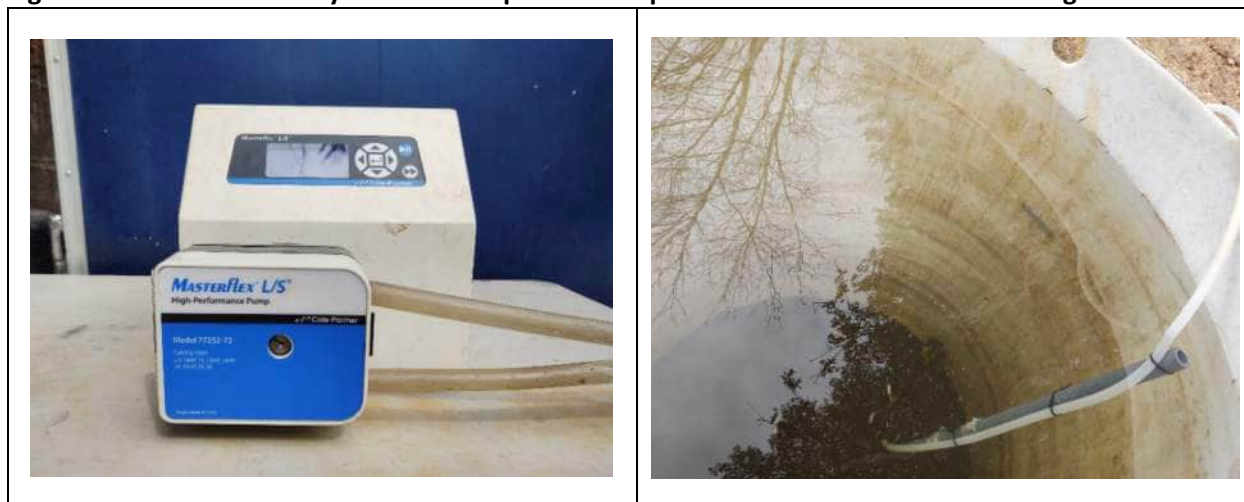
Figure 2.21: Peristaltic Recycle Feed Pump and Adsorptive Filter Backwash Water Storage Tank
