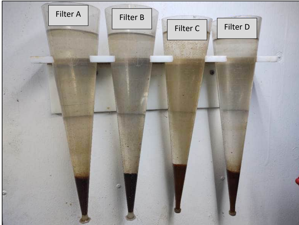
Figure 3.10: Photo of Imhoff Settling Cones
