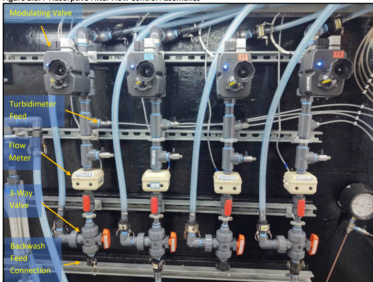
Figure 2.17: Adsorptive Filter Flow Control Assemblies
