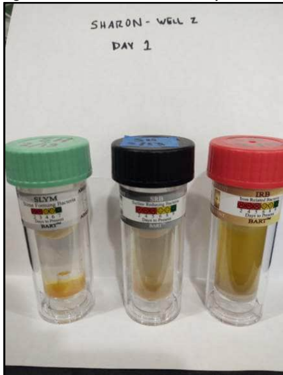
Figure 3.01: Well 7A BART Test, Day 1
