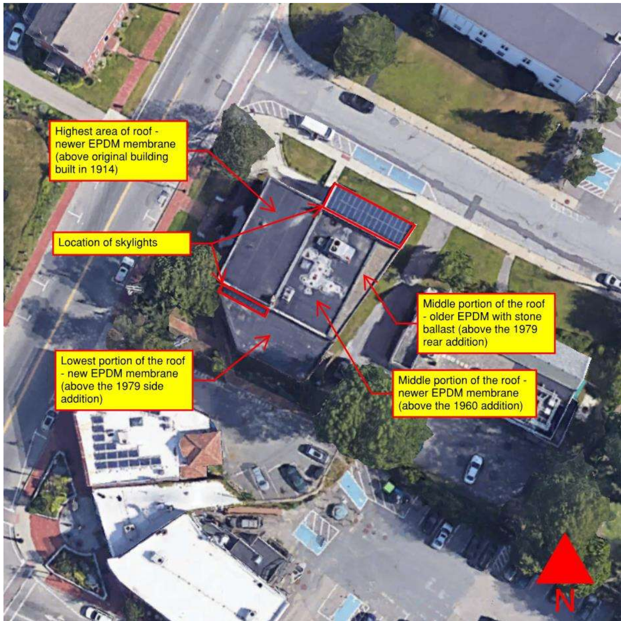
Figure 2 - Google Earth map 3-1: Building roof with notes (image taken prior to membrane replacement)
