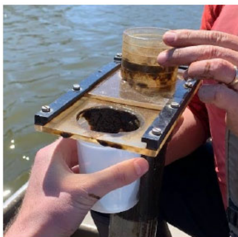
Figure A. Willner-type Coring Device in Use
