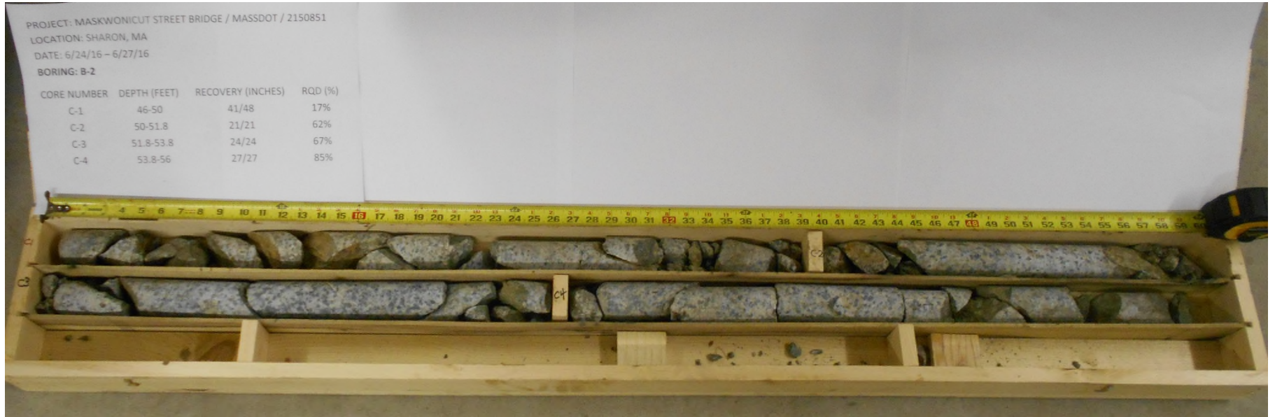
Top Row: Boring B-2, Core C-1 & C-2 Second Row: Boring B-2, Core C-3 & C-4
