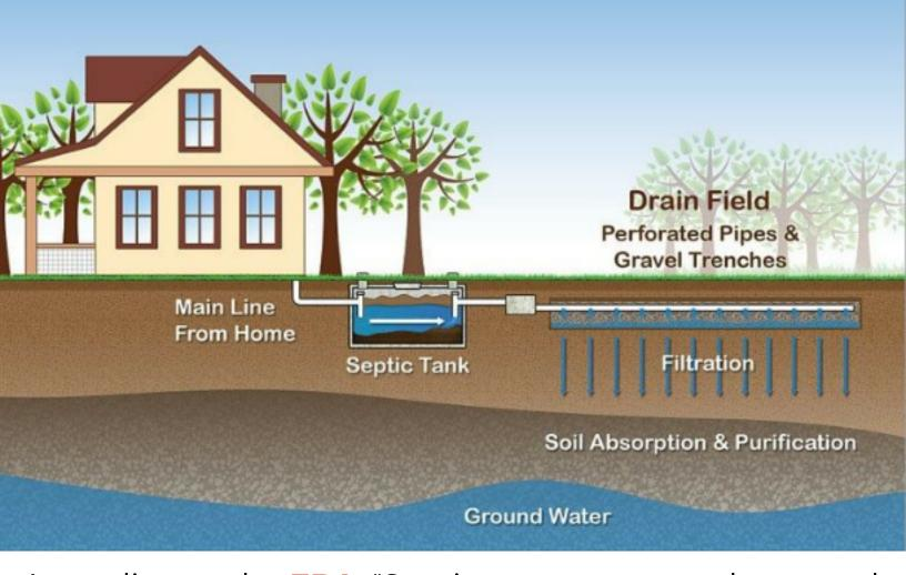
According to the **EPA**: "Septic systems are underground wastewater treatment structures [...] They use a combination of nature and proven technology to treat wastewater from household plumbing produced by bathrooms, kitchen drains, and laundry."
